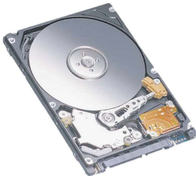
The disc of this hard drive moves from 5400 to 7200 times in a second
