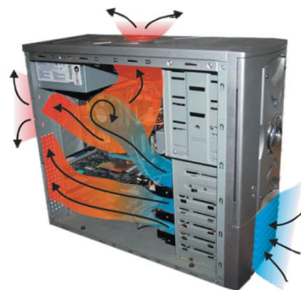
Proper airflow inside the computers must be ensured
